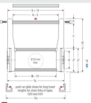
Calculating the cable carrier width
