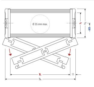
Calculating the cable carrier width
