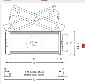
Calculating the cable carrier width
