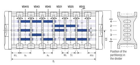
$\mathring{\vec{\textit{ll}}}$  Standard height separation with aluminum profile 11 × 4 mm.
