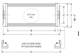
Calculating the cable carrier width
